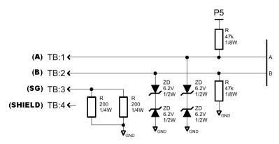
Figure 4: RS485 Interface Circuitry Schematic
